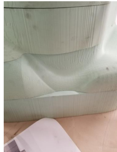
Figure 2 Ensure that no offsets are predetermined in CNC cuts to account for misalignment
