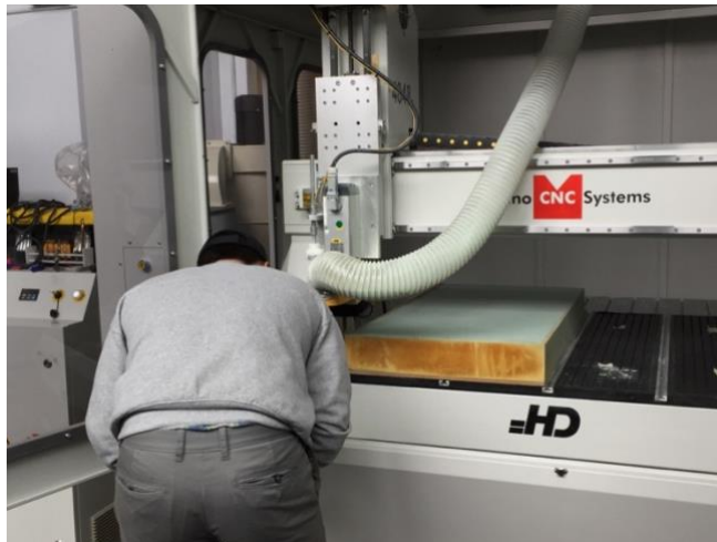
Figure 2 Ensure that no offsets are predetermined in CNC cuts to account for misalignment
